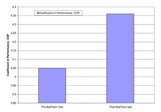
Chart 3C - Comparison of COP of Chiller 3 resulting from BallTech installation
